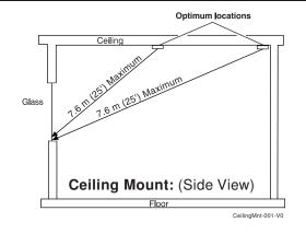
NOTE: If the device is ceiling mounted, the end with the hole (Microphone end) should face the protected glass.
