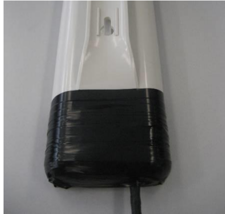
Figure 2-9 Second Layer-Electrical Tape
