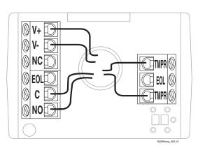
Normally Open Loop/No EOL Resistor
