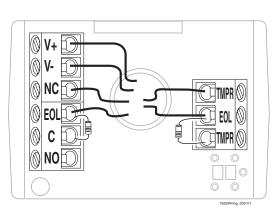
Normally Closed Loop/With EOL Resistor
