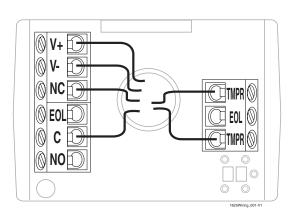
Normally Closed Loop/No EOL Resistor
