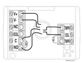
Normally Open Loop/With EOL Resistor
