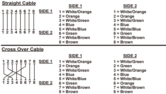
Figure A-1: Straight-Through and Crossover Cable
