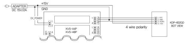
@ Connect pin no. 1(+13V) and no. 2(GND) of On LOB\_IN or LOB\_OUT PORT of KVS-A4P/A8P to +13V and GND of the doorphone in parallel.
