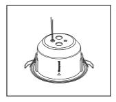
4. Push the loudspeaker to the ceiling hole using the spring, then the loudspeaker will be fixed automatically.
