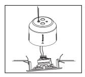
3. Align the slot of the back dome to the right place, and fix it. For LM2-PCP06A, please ignore this step.
