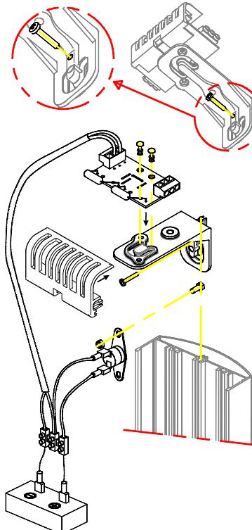
In order to maintain optimal performance in environments with low temperatures and condensation risk, **each tower must be equipped with one heater per beam unit, and a single thermostat switch.** I.e.: a tower containing 4 beam units will require 4 heaters and 1 thermostat switch. For large installations it may be necessary to run the beams and heaters on separate power loops, unless PSU's are installed in each tower.
