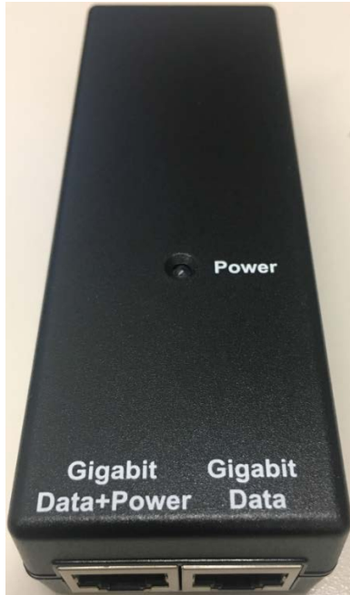
Figure 19 -20 to 32 VDC Power Injector interfaces
