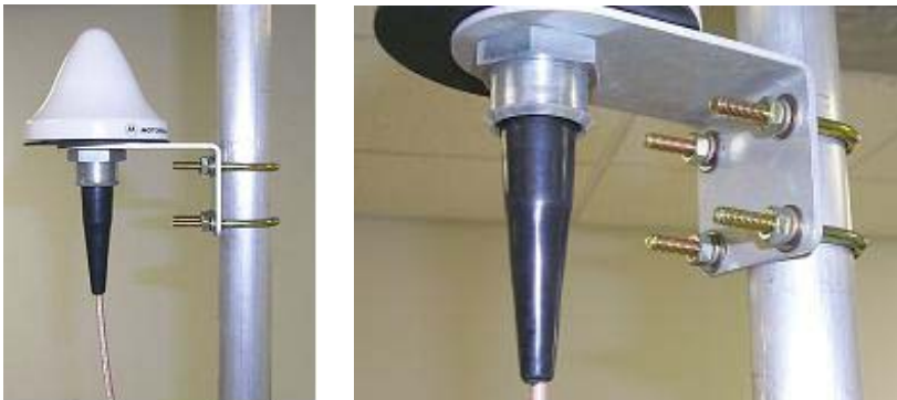
Figure 45 GPS antenna mounting
