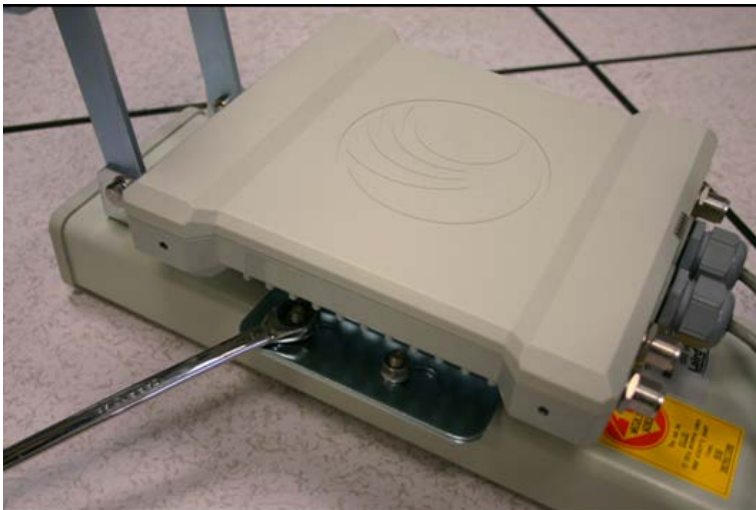
Figure 104 Lower bracket attached to AP antenna
