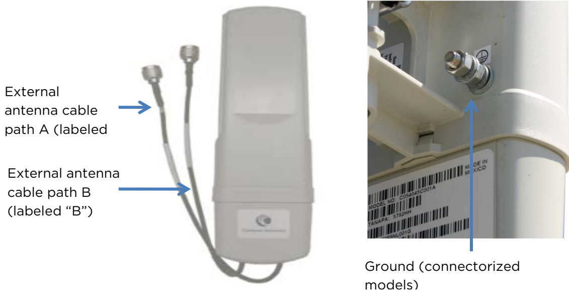
Figure 10 PMP/PTP 450 Series – SM/BH Connectorized interfaces
