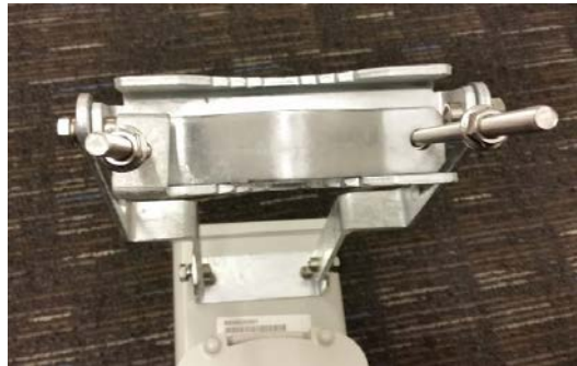
Figure 92 Assembled upper bracket connected to AP antenna
