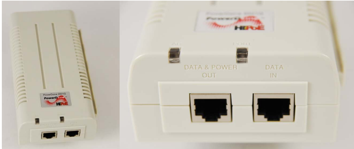
Figure 18 -48 V DC Power Injector interfaces
