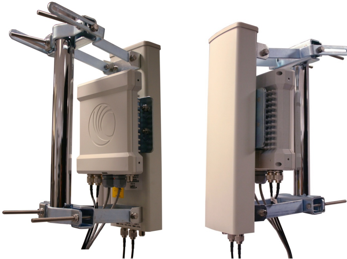
Figure 105 Mounted PMP 450 AP and antenna assembly, viewed from back and back
