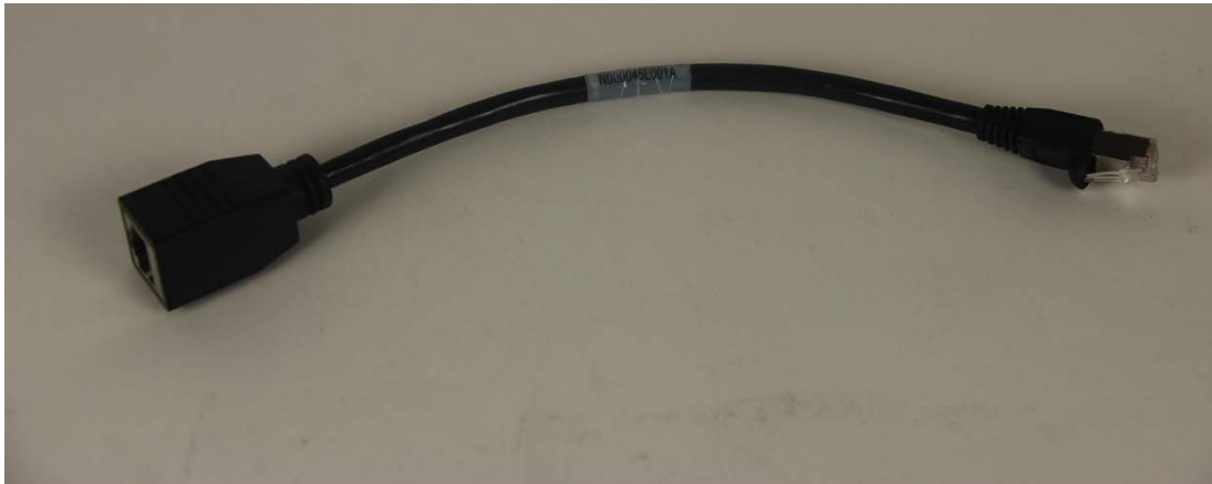
Figure 40 CMM4 56 V power adapter (dongle)
