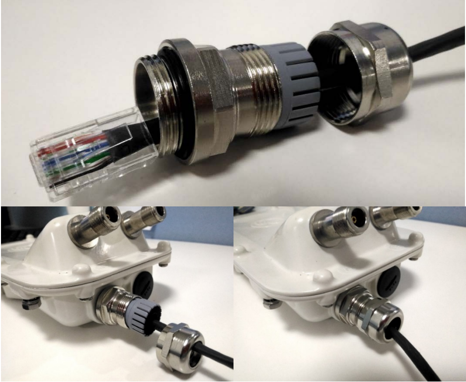
Figure 126 Ethernet cable gland for PMP/PTP 450i Series
