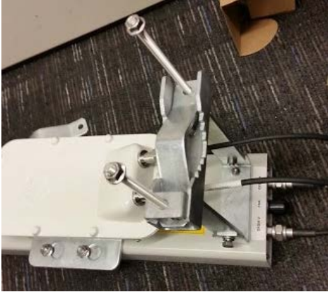
Figure 94 Lower bracket attached to AP antenna
