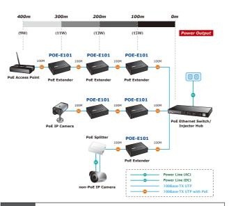
1. Per POE-E101 will take 2 watts maximum for the system itself, please check the total power consumption of your 802.3af PD and the POE-E101 before you make the daisy-chain connection. If the overall power consumption is overloaded, the local PSE could shutdown the whole power system.
