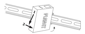
Step 3: Check the DIN-Rail is tightly on the track.
