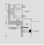
Accessories are available in a clear aluminum or black anodized finish. Verify length of magnetic lock before ordering mounting accessories.
