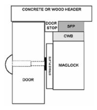
Sample Stop Filler Plate (SFP) and Concrete/Wood Bracket (CWB) combination
