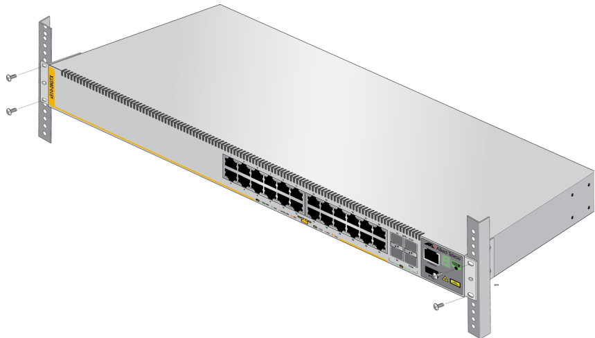
Figure 21. Mounting the Switch in an Equipment Rack
