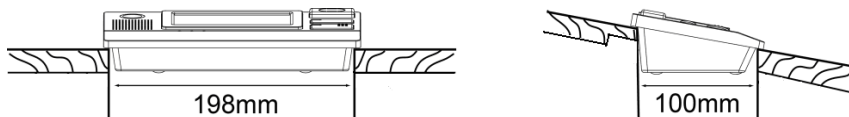
Figure 4 Schematic Diagram of Creating a Slot for Seating the NPM (Level Surface)
