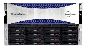
T-Series hybrid flash arrays combine the performance of flash memory and the economics of hard disk drives to deliver an efficient, hybrid storage solution. Ideal for applications that require cost-effective flash performance, IntelliFlash hybrid flash arrays offer exceptional value for storing and managing your secondary and backup data. The arrays come in various configurations that enable customers to dial up the flash:disk ratio to balance performance and economics as required.
